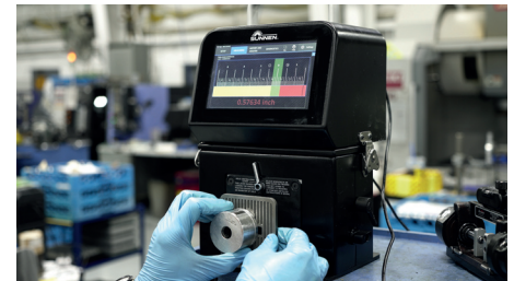
Using the new PGE-6000 digital gage, operator checks the bore diameter on the honed workpiece to be certain it is within tolerance
