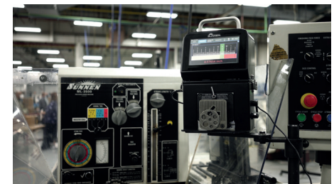
Kamatics places the Sunnen bore gauges on the shop floor next to honing stations for in-process measurement, as well as final inspection. Operators cite the portability, large range, high repeatability, and high accuracy as advantages of the PGE gauges
