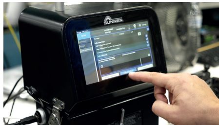
Sunnen's new PGE-6000 digital bore gauge incorporates a touch screen display, allowing quick and easy adjustments to the gauge settings
