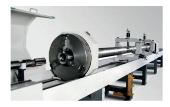
The **rotation device** prevents axis misalignment and guarantees a better bore geometry.
